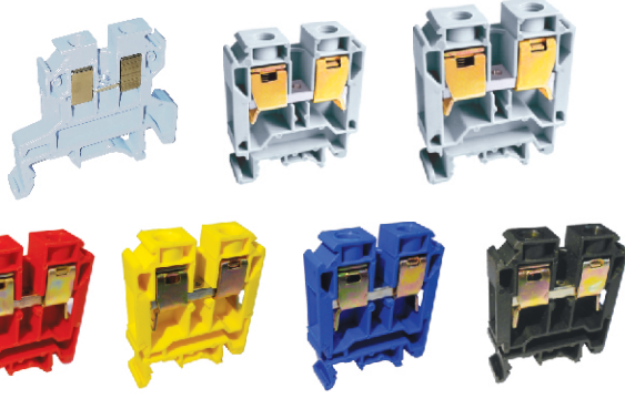
PB SERIES (With BRASS CLAMP) 1.5mm 2 - 35mm 2 , 750V AC
